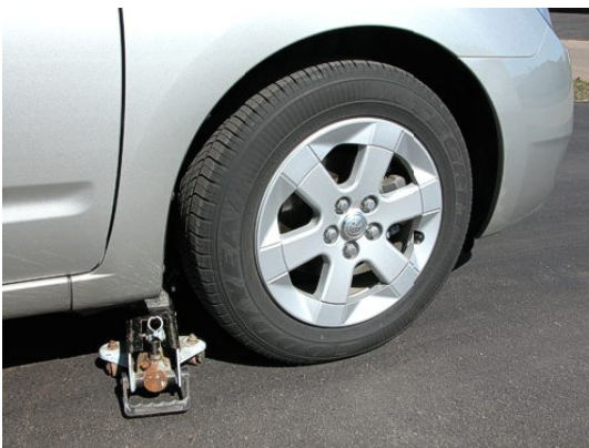
Lift location, before using the jack.
